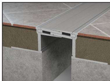
All metal floor expansion joint for exterior and interior use, allowing expansion and contraction of the joint as well as vertical movement and unlimited shear movement. For all types of finishes: screed, natural stone, cast stone, marble...
